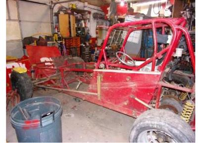
porta-power wizardry will correct that. No surprise broken welds or cracks. A basic Rust~olum tune up should have it in tip top shape. One thing he is going to change is the pan-hard bar set up. He likes a basic J-bar with a left side frame mount to the right side rear-end mount. That thing must have had 3 lbs. of Duzs buttons in it. But it now sits naked and ready to have the '37 Ford slant back body fitted to it. Next is getting the '37 in the shop and get it stripped down.
